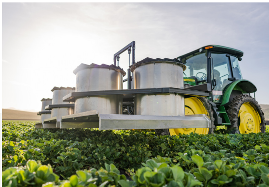
Strawberry growers use bug vacuums in their fields as part of their integrated pest management strategy.
